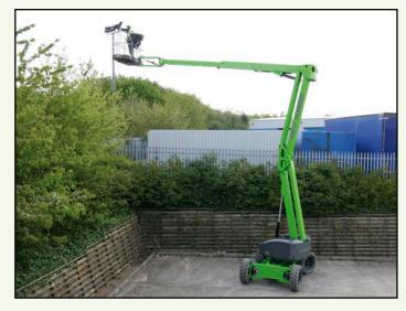
The HR17 Hybrid 4x4 also incorporates ToughCage and SiOPS™ technologies. A touah impact resistant composite base and larger cross-section steel give the ToughCage strength and durability, while **SiOPS™** offers additional operator protection.
